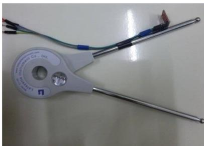
Figure 5: Goniometer with Accelerometer.
