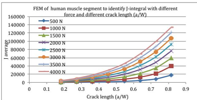
Figure 6: Different applied loads with different laceration lengths
