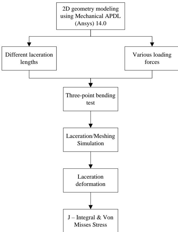
Figure 2: Block diagram that been used to obtain strain energy release rate and von Mises stress
