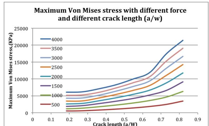
Figure 8: Von Mises stress with different applied load and different crack length
