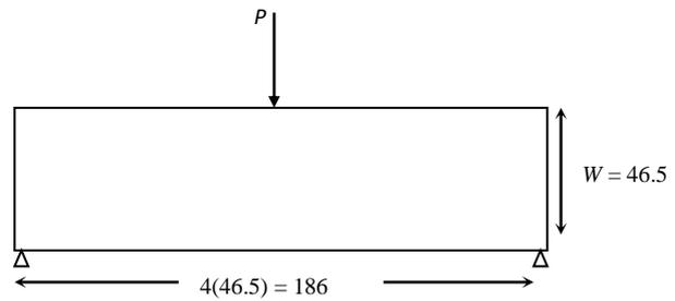
Figure 3: Configuration of three-point bending test on a human muscle
