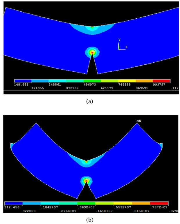
Figure 7: Different applied loads with a laceration length of 0.0296 m (a)  $P = 500$  N, (b)  $P = 3000$  N
