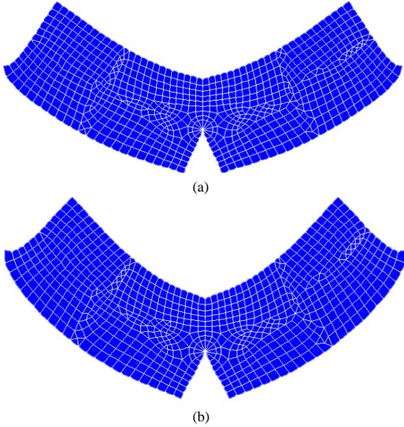
Figure 5: Different applied loads with a laceration length of 0.0296 m (a)  $P = 1500$  N, (b)  $P = 3000$  N
