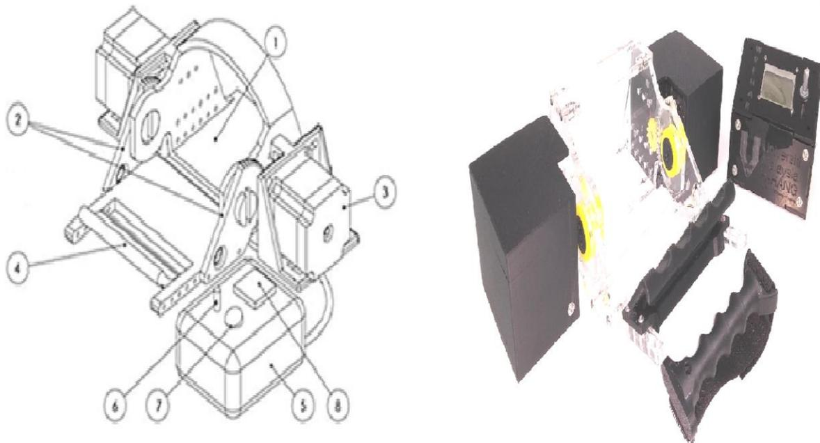
Figure 1: *Right*-Illustrated an embodiment of the WRist-T device. *Left*-The prototype of the wrist rehabilitation therapy (WRist-T) device. Notes: Description of the reference numerals used in the accompanying drawings according to the WRist-T device; (1) channel; (2) platform arm; (3) motor; (4) hand support; (5) controller; (6) toggle switch; (7) power button; (8) LCD display.
