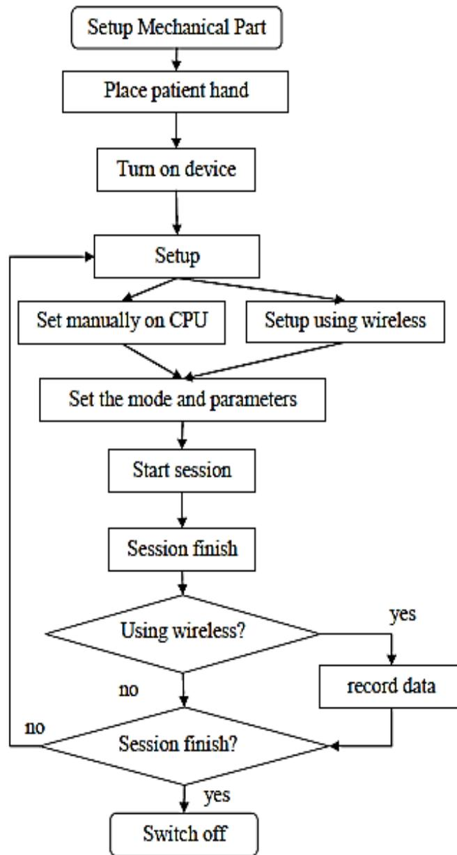
Figure 3: The flowchart of the WRist-T device function.
