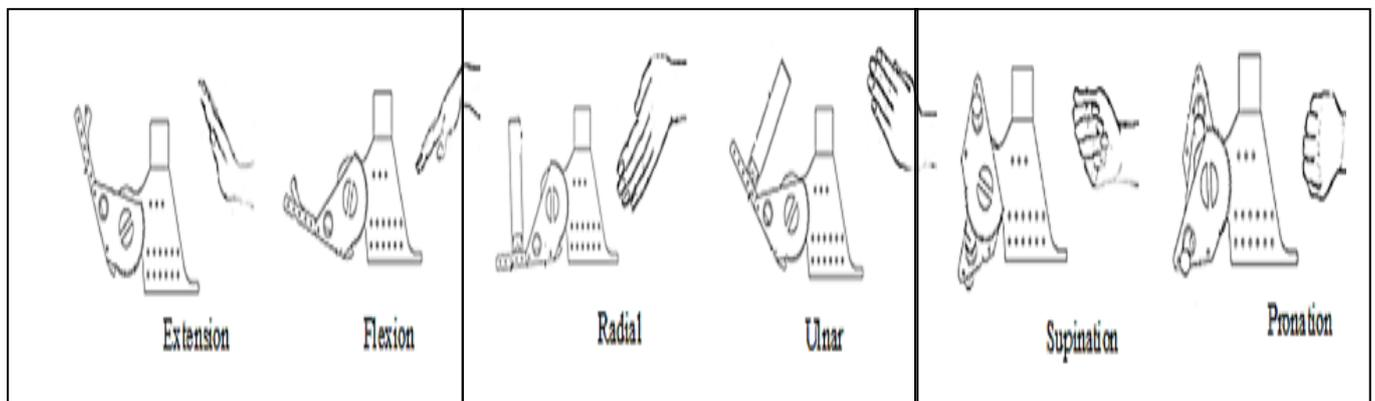
Figure 2: A perspective views of the device in an embodiment to give (a) Motion foreextension/flexion; (b) Radial/ulna deviation; and (c). Supination/pronation of the wrist.
