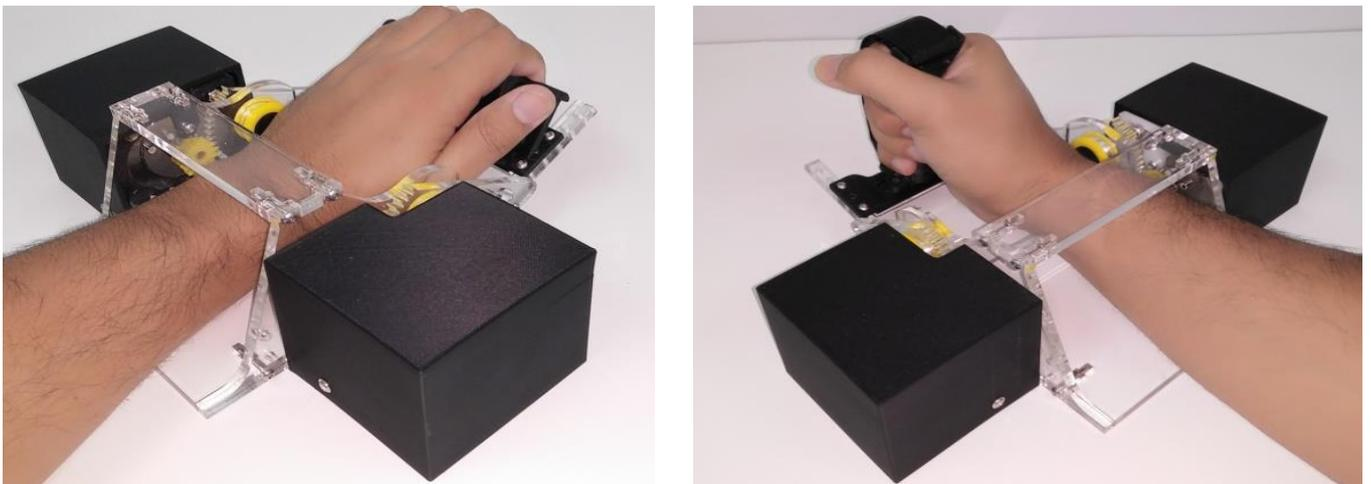
Figure 4: A 3D printed prototype of WRist-T device tested to an ischemic stroke patient. The figure shows details the example wrist of motion on extension/flexion and radial/ulnar deviation exercise.
