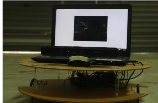
Figure 7: The mobile scanner
