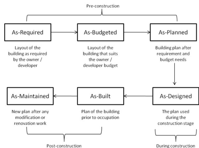
Figure 1: Stages of various planning involves in constructing and maintaining/monitoring a building, where the as-is plan is located between as-built and as-maintained [1]
