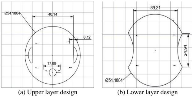
Figure 5: Drawing of the platform designed using AutoCAD 2016
