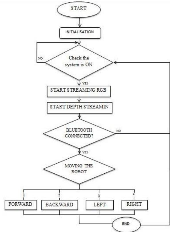
Figure 4: The flowchart of the mobile scanner
