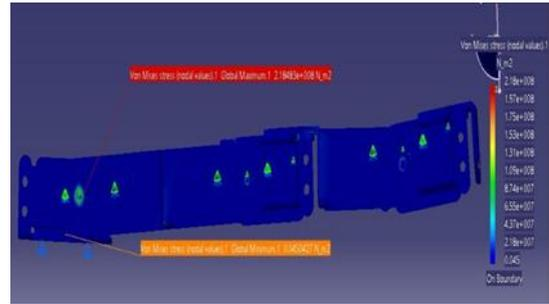
Figure 4: Result of Von Mises stress on the robot arm
