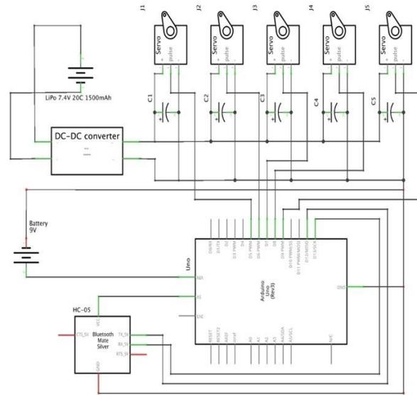
Figure 9: Schematic diagram of the robot arm
