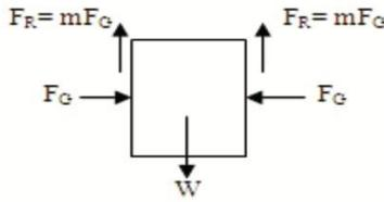
Figure 7: Free body diagram of the target object in the gripper
