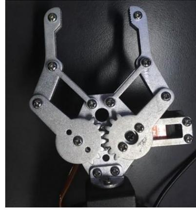
Figure 8: Hardware of gripper
