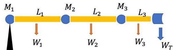
Figure 6: Free body diagram of the robot arm
