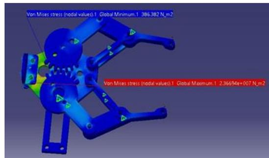
Figure 5: Result of Von Mises stress on the robot arm
