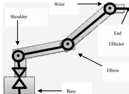
Figure 1: Free body diagram of the 4DOF robot arm
