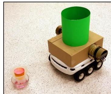
Figure 2: Mobile robot equipped with a pair of gas sensors [13].
