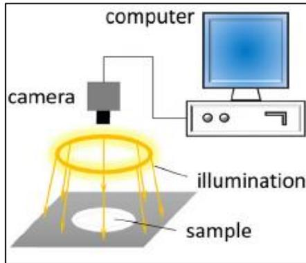
Figure 2: The fundamental of machine vision workstation
