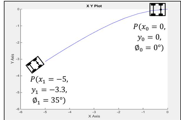
Figure 19: Reverse right parking plotted in XY-graph
