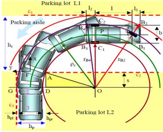
Figure 3: Geometry of collision-free reverse perpendicular parking manoeuvre [5]
