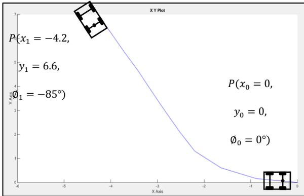
Figure 15: Reverse left parking plotted in XY-graph
