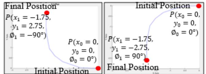
Figure 8: Graph for reverse left (3) and right (4) motion
