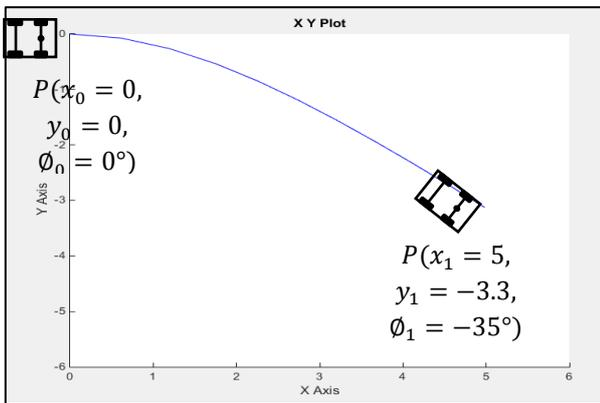
Figure 17: Forward right parking plotted in XY-graph
