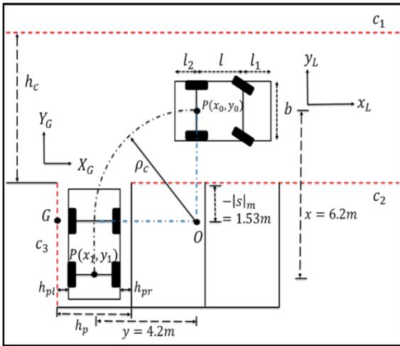
Figure 5: Geometry of perpendicular reverse right
