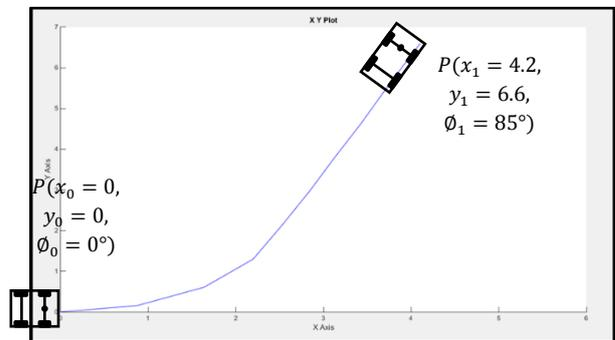
Figure 13: Forward left parking plotted in XY-graph
