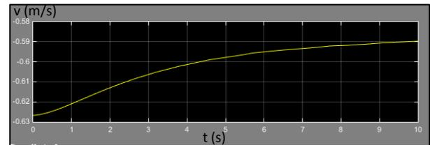
Figure 20: Speed of the reverse right parking
