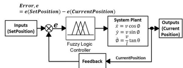
Figure 9: General control block diagram of closed-loop simulation
