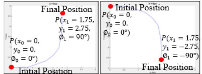
Figure 7: Graph for forward left (1) and right (2) motion
