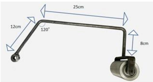
Figure 3: Dimensions of the roller arm
