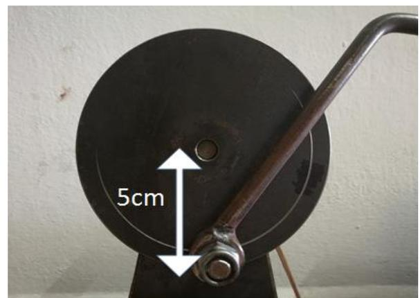
Figure 6: Distance between the joint of roller arm to the centre point of driving disc.
