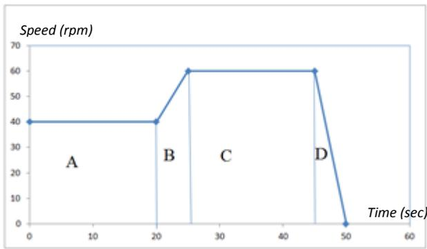
Figure 7: Desired conching process output profile.
