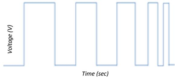
Figure 9: PWM input signal for segment B (acceleration)
