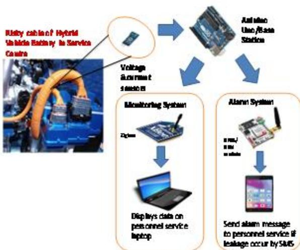
Figure 2: System architecture design
