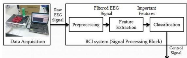
Figure 1: Block diagram of BCI system
