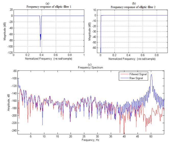
Figure 2: (a) Frequency response of Elliptic band stop filter with 50 Hz cut-off frequency; (b) Frequency response of Elliptic high pass filter with 1 Hz cut-off frequency; (c) Frequency spectrum of raw EEG signal vs filtered EEG signal
