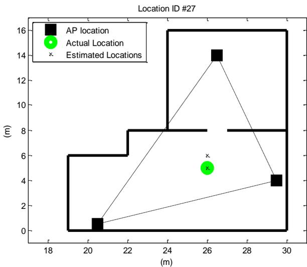
Figure 10: The positioning accuracy of the positioning system on using LKF filter
