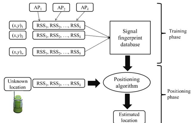
Figure 1: A typical flow of the wireless positioning system based on fingerprinting technique
