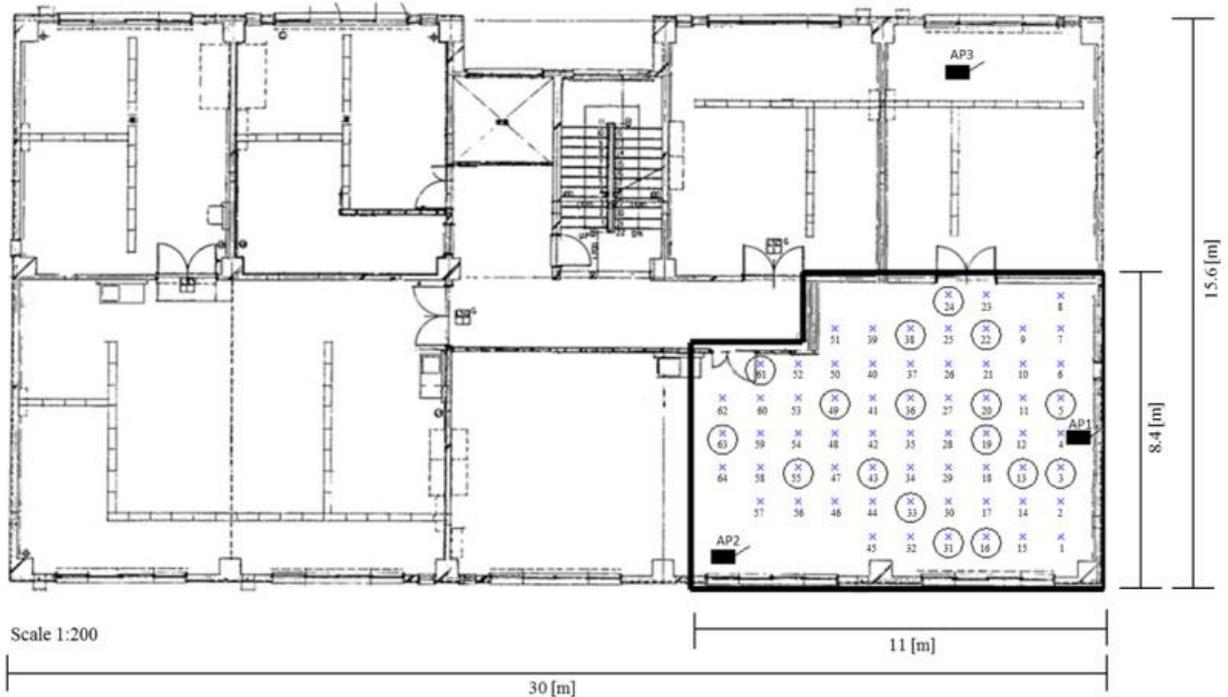
Figure 5: Experimental area showing the location of the WiFi Access Points (AP) and signal fingerprints database [8]
