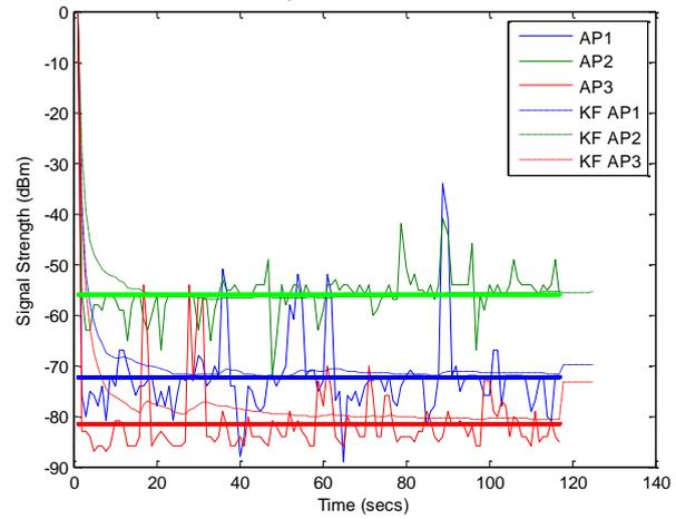
Figure 6: Effectiveness of Linear Kalman Filter towards prediction of the WiFi signal in a stationary location
