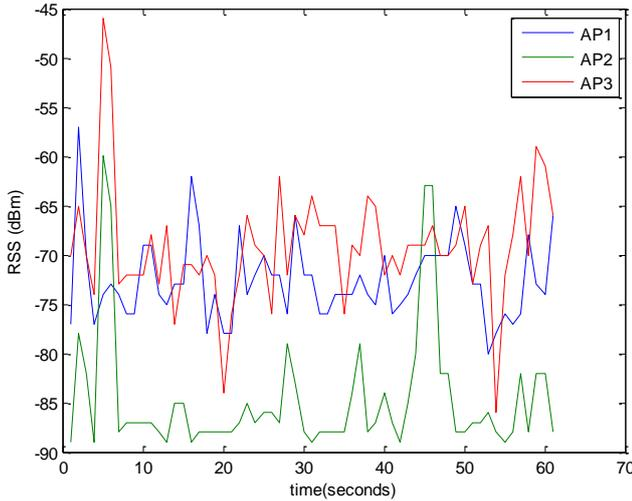
Figure 2: An example of the WiFi signal fluctuation where the mobile robot stays stationary over some period of time.
