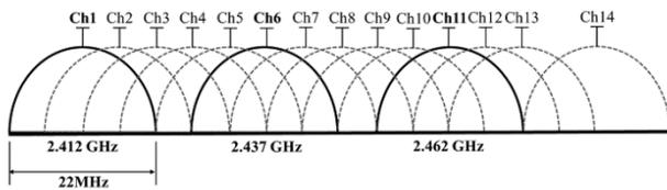
Figure 3: The 802.11 WiFi channels in the 2.4GHz spectrum
