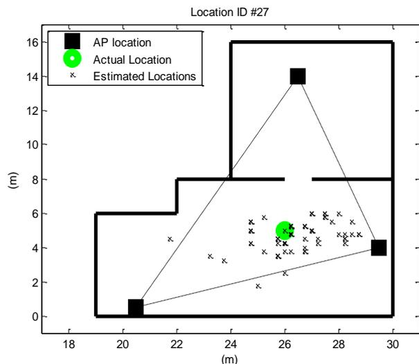
Figure 8: The positioning accuracy of the positioning system on using raw data
