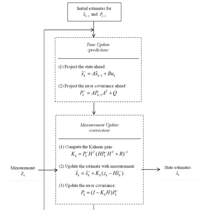
Figure 4: Linear Kalman Filter algorithm
