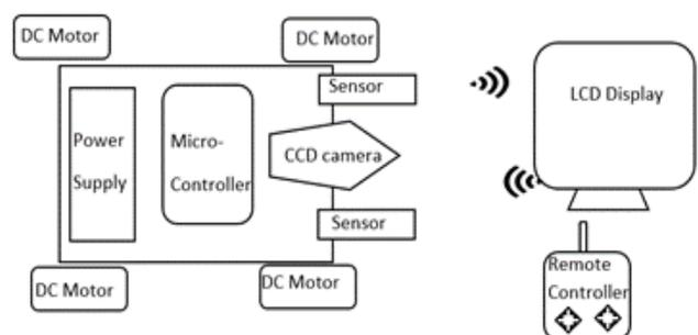
Figure 2: Mobile robot architecture.
