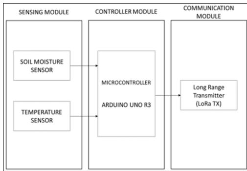
Figure 1: Transmitter (Node) Block Diagram of the System
