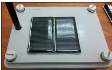
Figure 7: Solar Panel attached to node box
