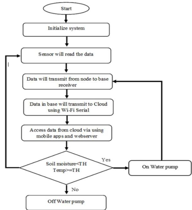
Figure 5: Automatic Irrigation Monitoring System Using Android Based Application Algorithm
