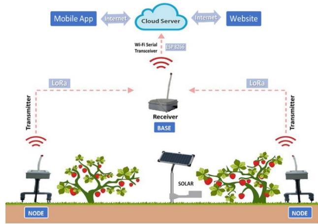
Figure 4: The Operation of the System
