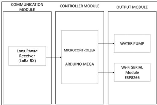
Figure 2: Receiver (Base) Block Diagram of the System
