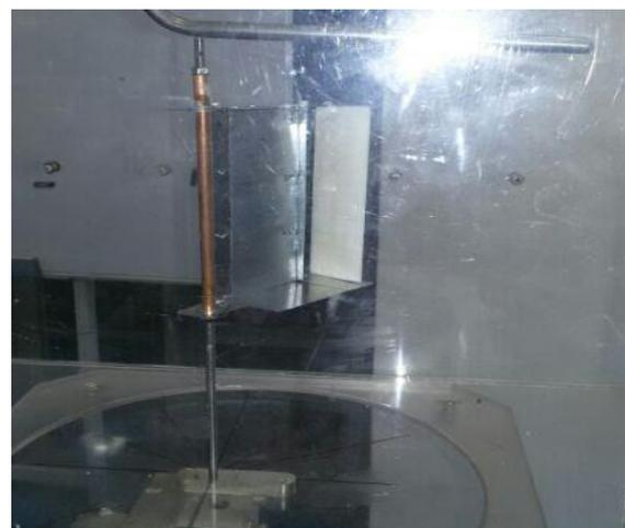
Figure 3: Experiment Setup of Combined Frame in Wind Tunnel
