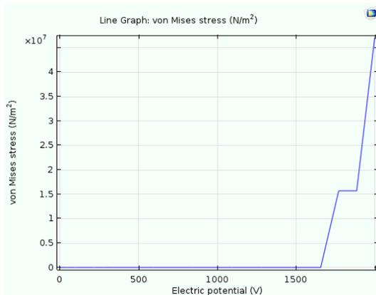
Figure 5: The stress versus electric potential for carbon grease electrodes graph.
