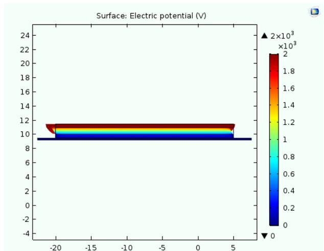
Figure 4: DE expansion with carbon grease electrodes
