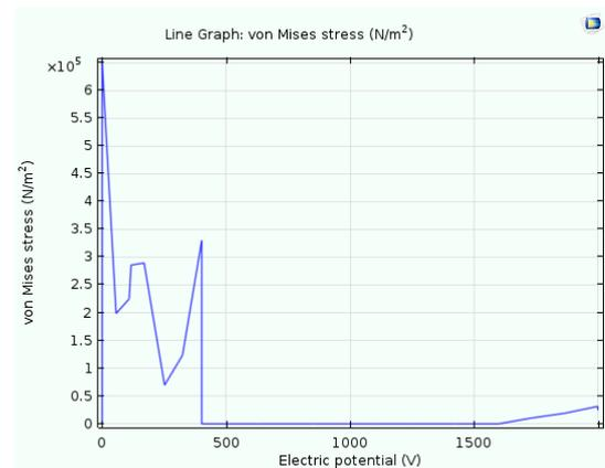
Figure 7: The stress versus electric potential for carbon powder electrodes graph
