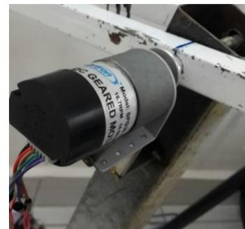
Figure 6: DC motor in place
