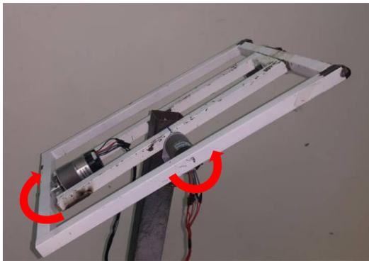
Figure 8: Dual axis rotations
