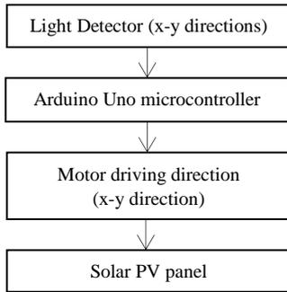
Figure 1: Block diagram of hardware implementation of dual-axis solar tracker
