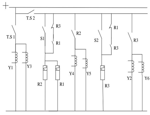
Figure 4: Solenoid circuit of miniature compressed air storage system
