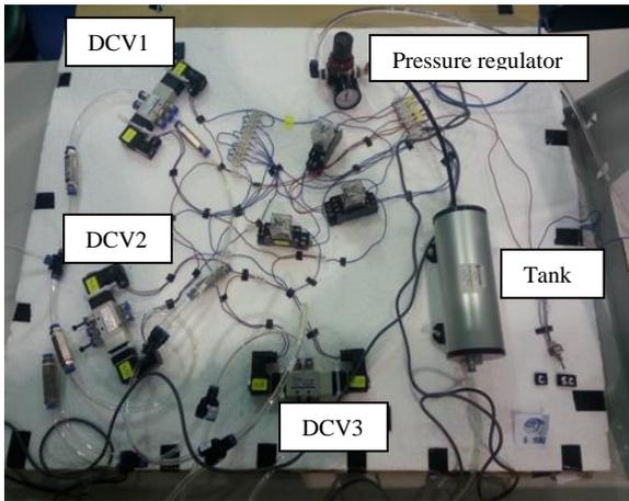
Figure 1: Pneumatic circuit of the compressed air storage system
