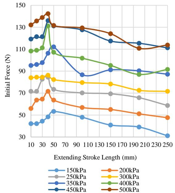
Figure 5: Extending piston stroke length (mm) versus Initial Force (N)
