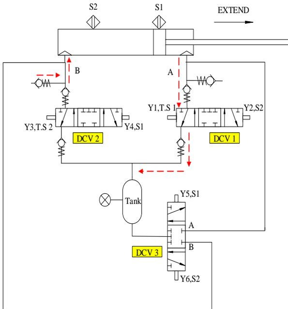
Figure 2: Extending piston of the miniature compressed air storage system
