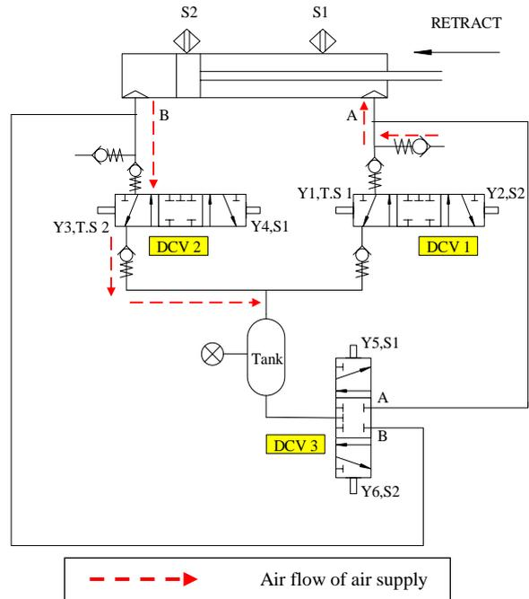
Figure 3: Retracting piston of the miniature compressed air storage system
