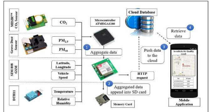
Figure 1: In-vehicle air quality monitoring architecture design.
