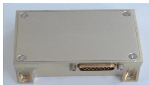
Figure 2: The RazakSAT magnetometer
