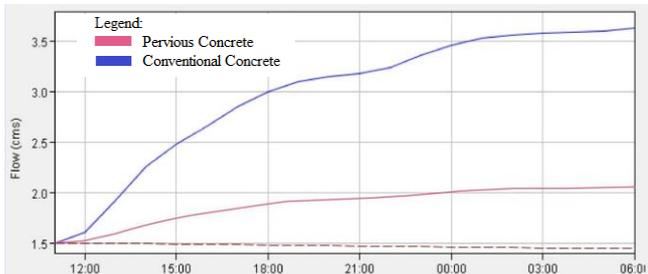
Figure 7: Summary of Flow (Pervious Concrete Road)
