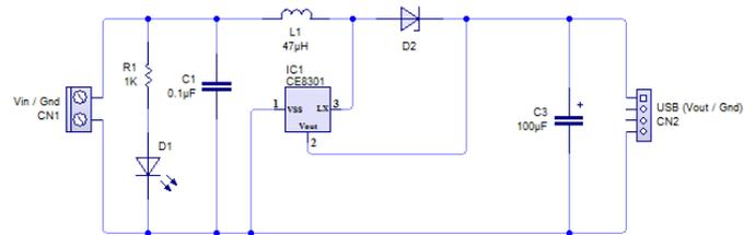
Figure 3: Step-up Boost Converter Schematic Diagram
