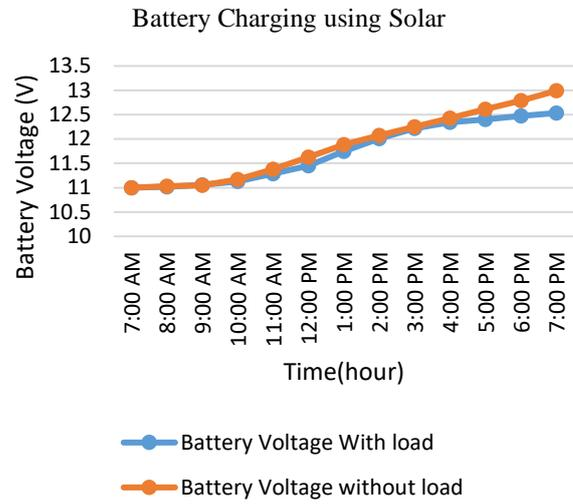
Figure 7: Battery charging using solar
