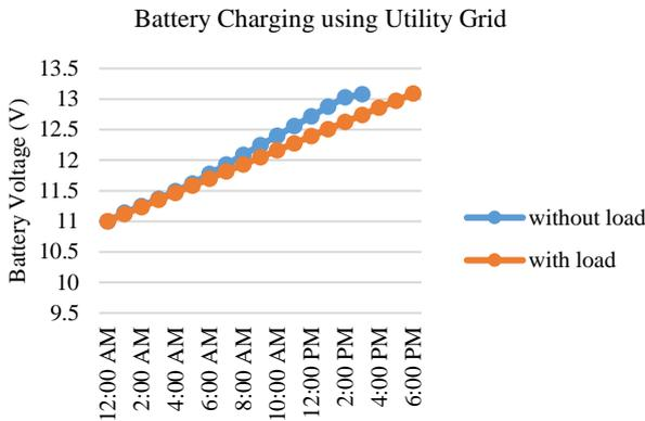
Figure 6: Battery charging using utility grid
