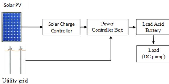
Figure 1: Block diagram of the proposed Hybrid Energy System
