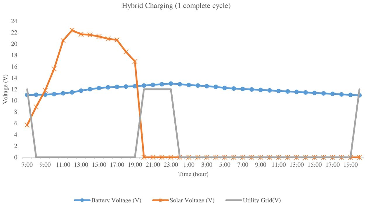
Figure 8: Battery charging using hybrid power sources
