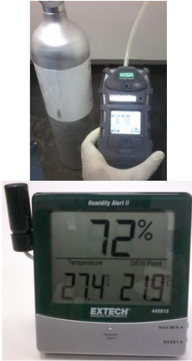
Figure 7: Altair 5x Multi Gas Detector and Humidity Alert II
