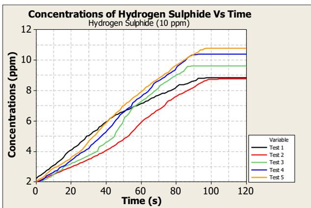
Figure 8: Graph of H<sub>2</sub>S concentrations (10 ppm) versus time
