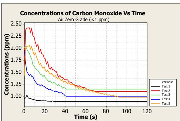
Figure 12: Graph of CO concentrations (<1 ppm) versus time
