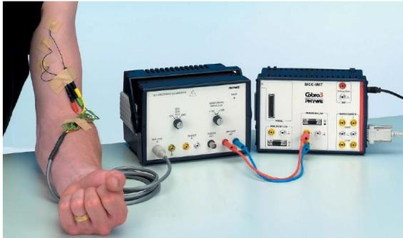
Figure 3: Bio amplifier PHYWE COBRA3
