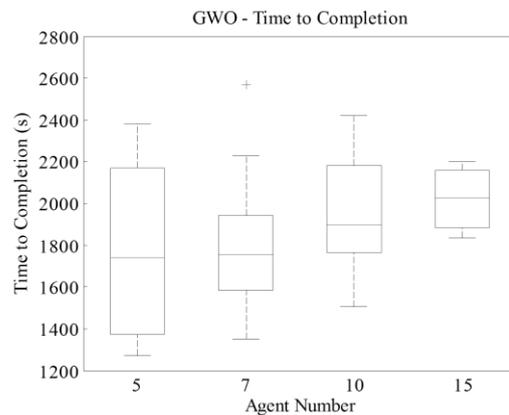
Figure 5: Time to completion with a different number of robots
