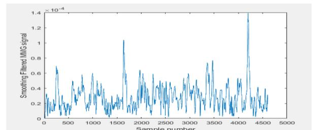
Figure 9: Final signal after rectified and smoothing
