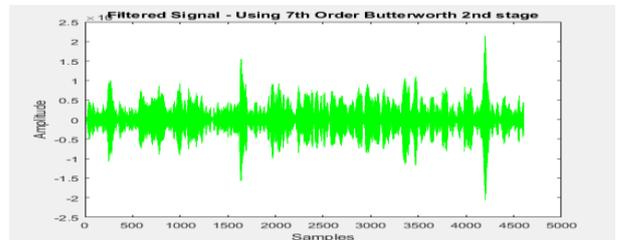
Figure 8: Signal after second stage of band pass filter
