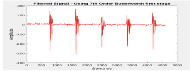
Figure 6: Signal after low pass filter
