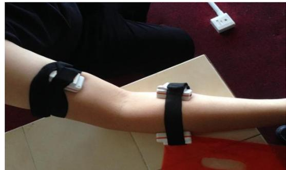
Figure 1: Position of triaxile Accelerometers in hand
