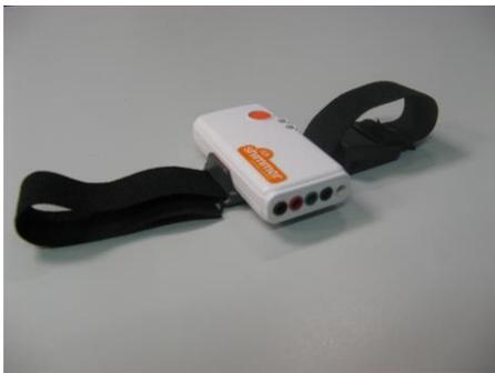
Figure 4: Shimmer3 EMG unit (ShimmerSensing)
