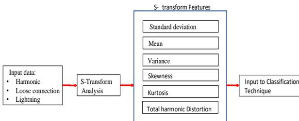
Figure 1: Features extraction module
