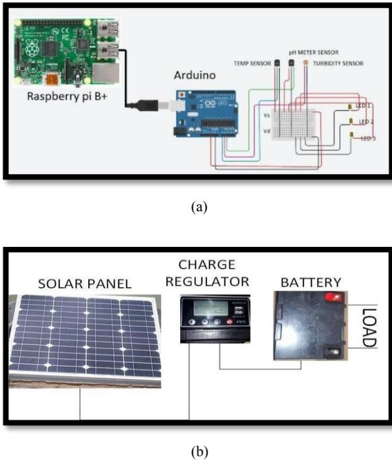
Figure 2: (a) Schematic diagram of the sensor module (b) Power supply consideration for the system
