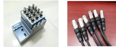
Figure 3: NI cDAQ-9174 and acceleration sensors
