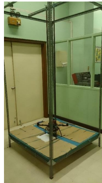
Figure 10: Payload Drop Test Rig
