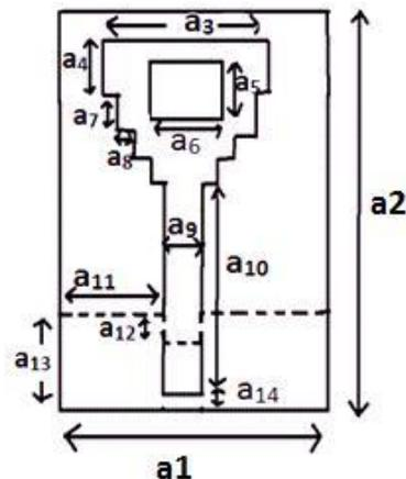
Figure 1: Sketch of the bidirectional antenna
