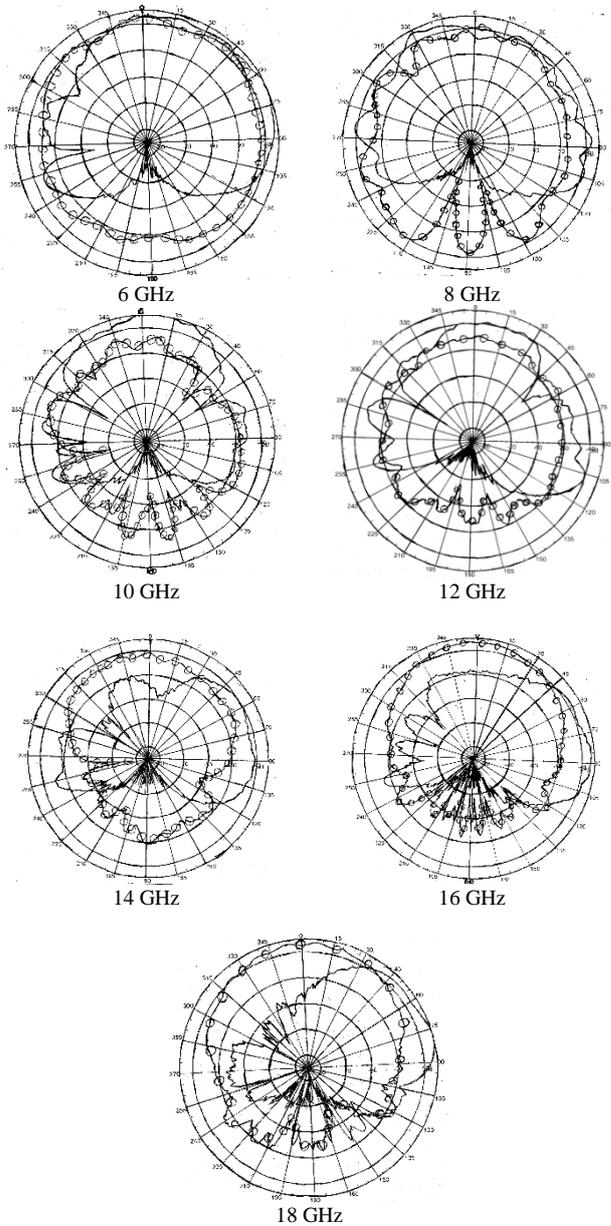
Figure 9: Radiation patterns (Unidirectional)
