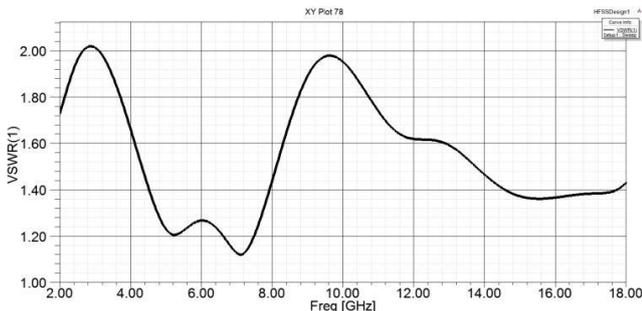
Figure 4: VSWR of bidirectional antenna
