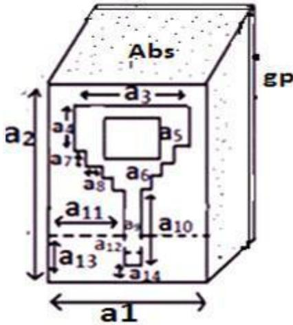
Figure 2: Sketch of the unidirectional antenna
