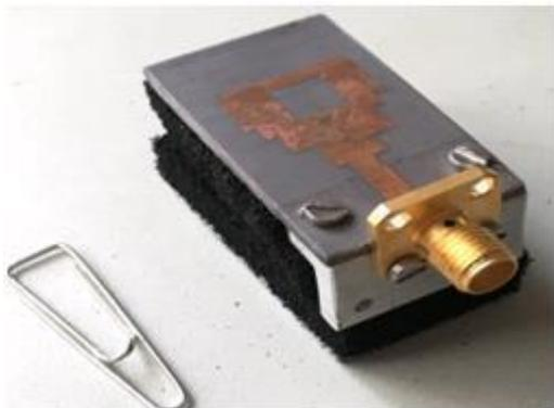
Figure 3: Photograph of the unidirectional antenna
