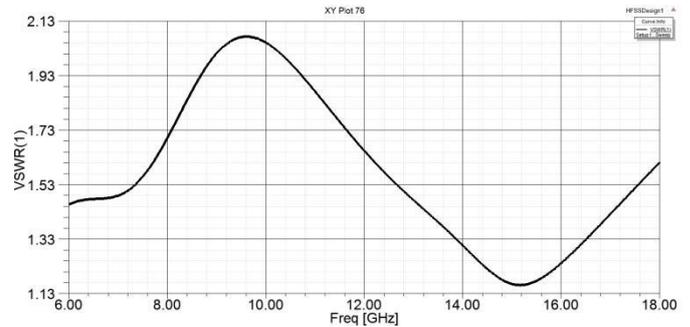
Figure 5: VSWR of unidirectional antenna
