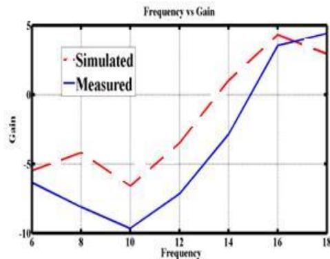
Figure 10: Frequency versus Gain of unidirectional antenna
