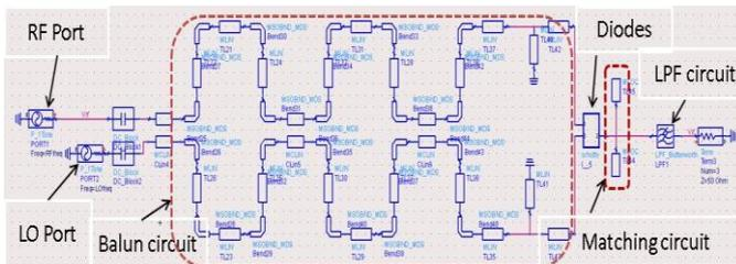
Figure 9: Schematic of single balanced mixer
