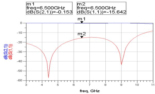
Figure 5: Low Pass Filter results
