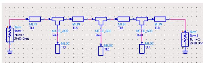
Figure 4: Schematic of Low Pass Filter
