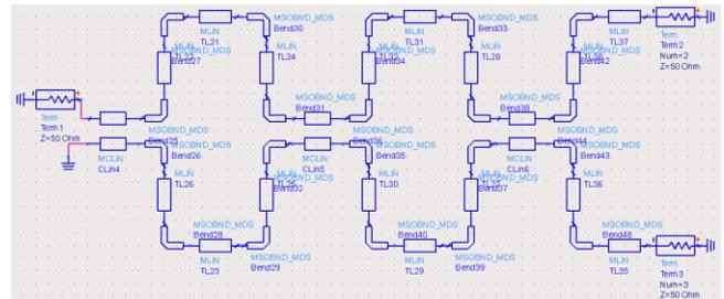
Figure 6: Schematic of Balun Circuit
