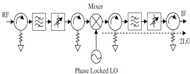
Figure 1: Typical diagram of the transceiver simulator [2].
