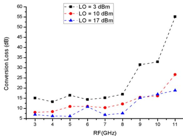
Figure 10: Simulated Conversion loss with various level of LO power
