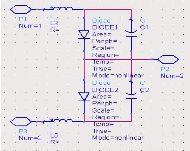
Figure 3: Schematic of Schottky diode
