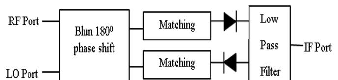
Figure 2: Equivalent single balanced mixer circuit.
