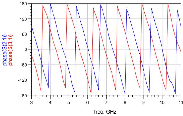
Figure 8: Phase response of the balun circuit for port 2 and port 3
