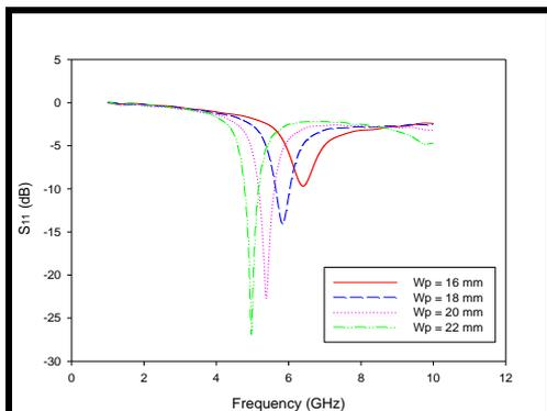
Figure 4: Optimization process for width of the patch
