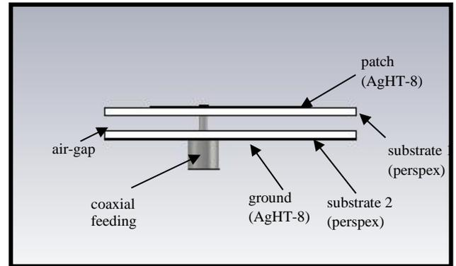
Figure 5: A cross-sectioned view of the stacked transparent patch antenna
