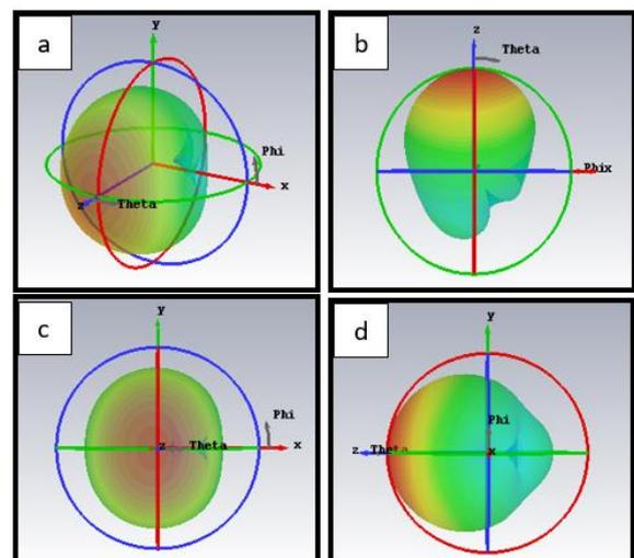
Figure 11: Simulated radiation pattern for a dual-stacked transparent patch antenna: (a) Perspective view, (b) top view, (c) front view, (d) side view.
