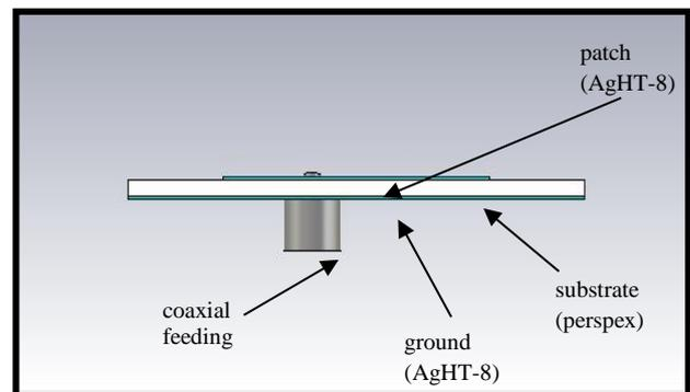
Figure 1 : A cross-sectioned view of the single transparent patch antenna
