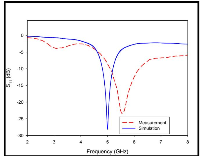
Figure 10: Simulated and measured results of return loss for a dual-stacked transparent patch antenna.
