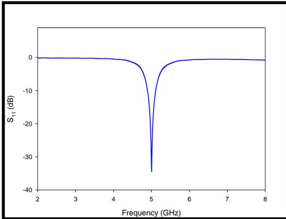
Figure 7: Simulated return loss of a single transparent patch antenna
