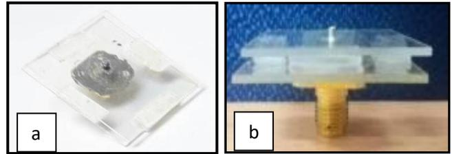
Figure 9: Prototype of dual stacked transparent patch antenna; (a) Front view and (b) side view.
