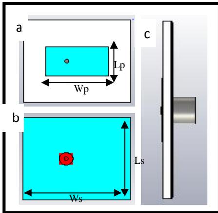
Figure 2: A single patch antenna: (a) Front view, (b) back view (c) side view
