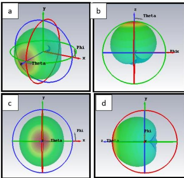
Figure 8: Simulated radiation pattern for a single transparent patch antenna: (a) Perspective view, (b) top view, (c) front view and (d) side view
