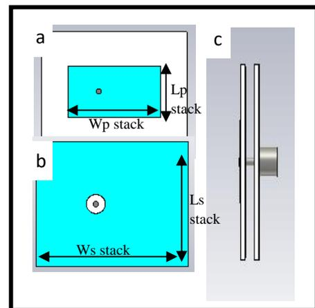
Figure 6: A dual-stacked patch antenna: Front view (a) Front view, (b) back view and (c) side view
