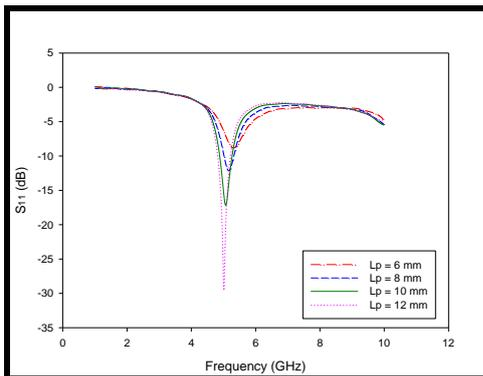
Figure 3: Optimization process for length of the patch
