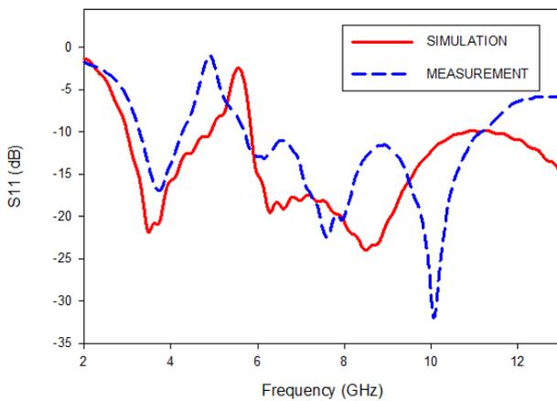
Figure 5 :  $S_{11}$  of the antenna during ON mode
