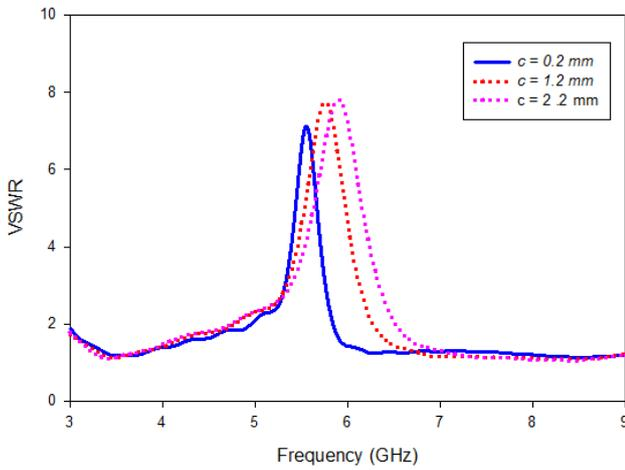
Figure 4 : VSWR of the antenna with variation values of  $c$
