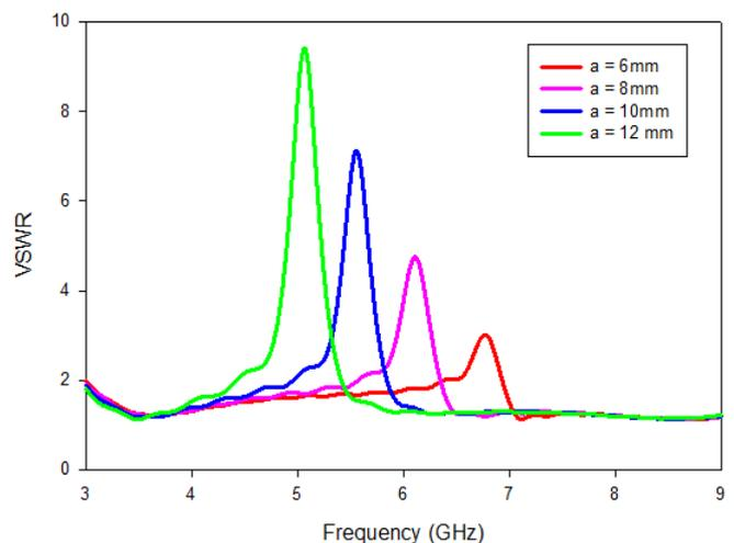
Figure 3: VSWR of the antenna with variation values of  $a$
