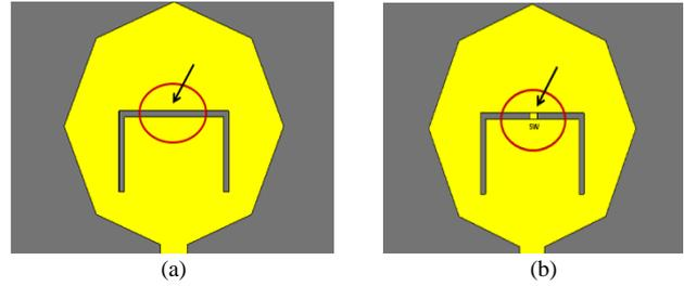
Figure 2: Switch integrated into the antenna (a) On mode (b) Off mode
