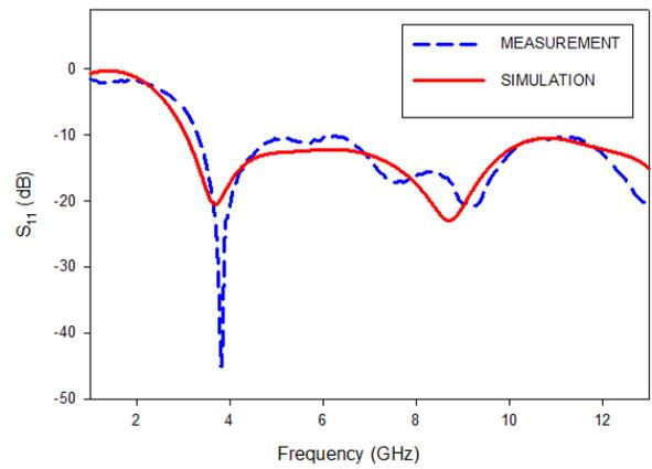
Figure 6 :  $S_{11}$  of the antenna during OFF mode
