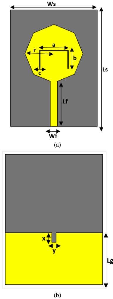
Figure 1: The configuration of the antenna (a) top view (b) bottom view
