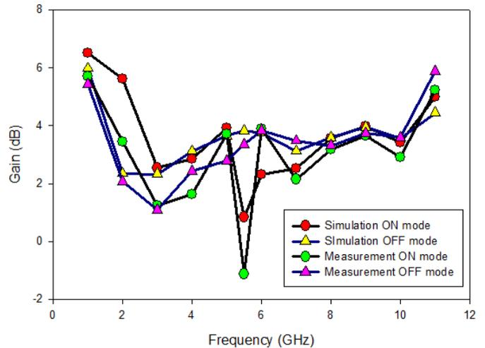
Figure 7: Simulated and measured antenna gain during ON and OFF mode
