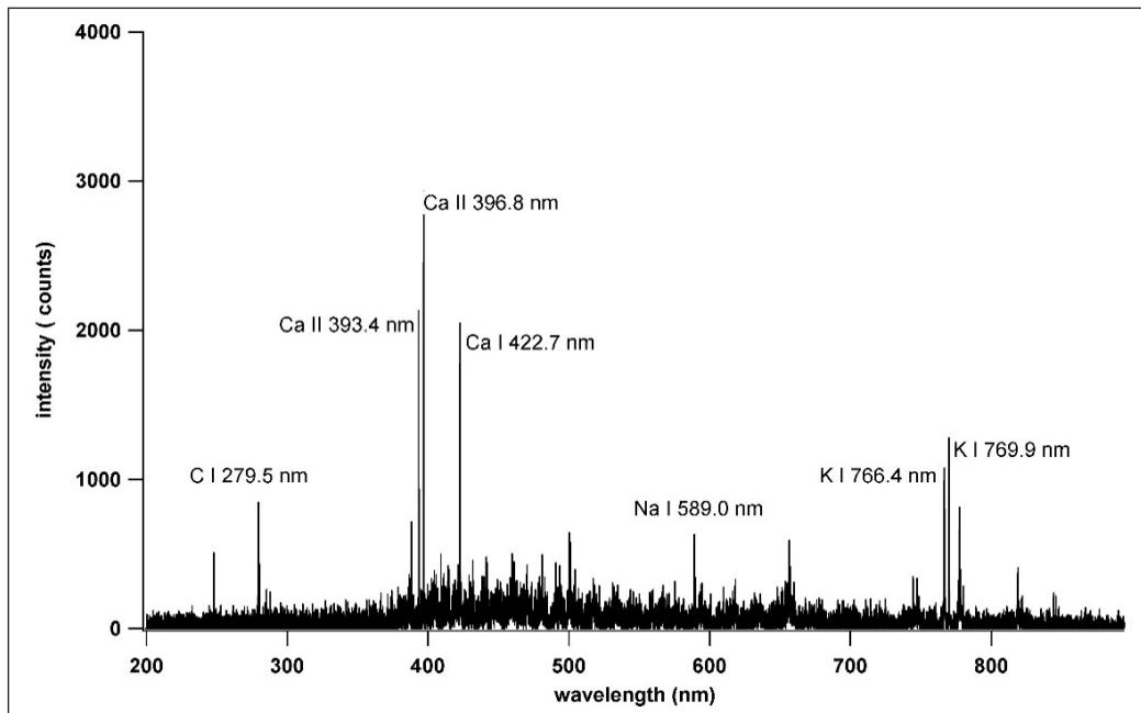
Figure 4(b). Spectrum of pectin made of horn shaped banana.
