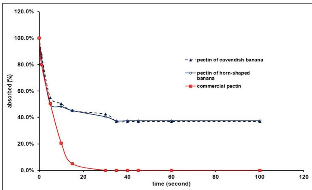
Figure 3. Pb I 405.7 nm emission intensity as a function of time after pectin introduction into the water which is containing 0.1 g  $PbCl_2$ .
