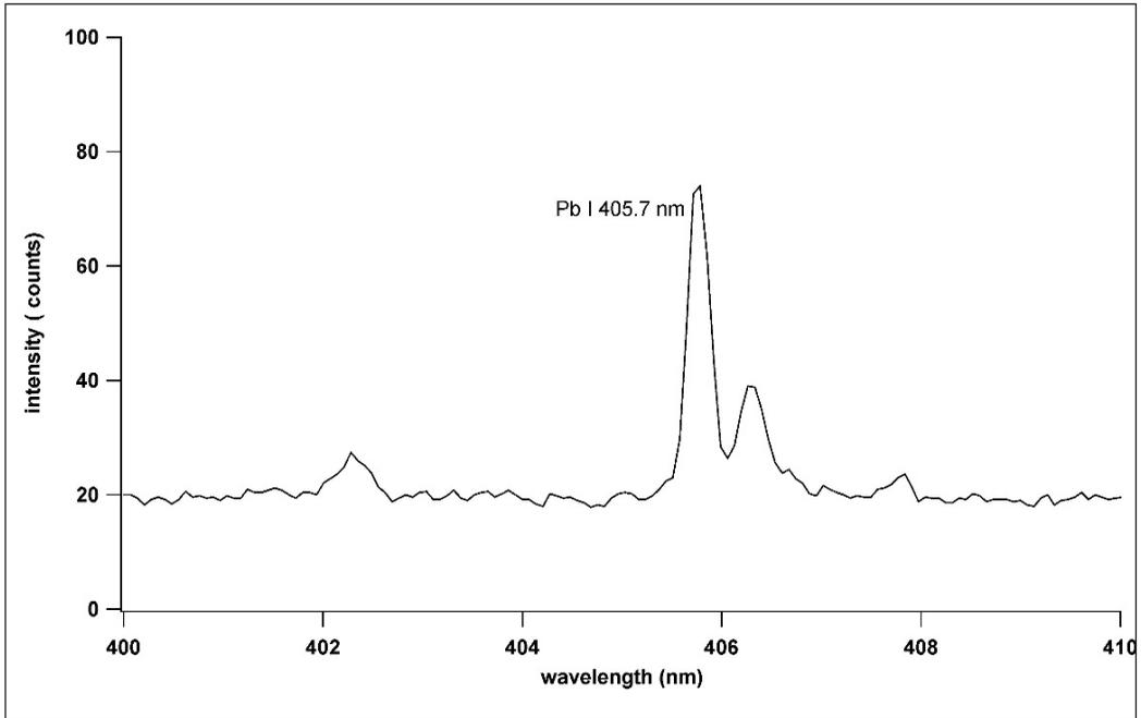
Figure 5(a). The effectiveness of Pb I 405.7 nm adsorption in liquid by using pectin and the spectrum of 40 ml H<sub>2</sub>O + 0.1 g PbCl<sub>2</sub>
