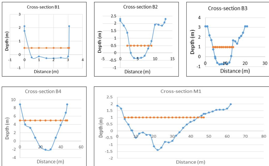
Figure 4. Five main river cross sections from the upper segment B1 to the lower segment at M1. The river cross section is shown by the blue lines, while red lines are the water depth at the time of measuring the cross sections.
