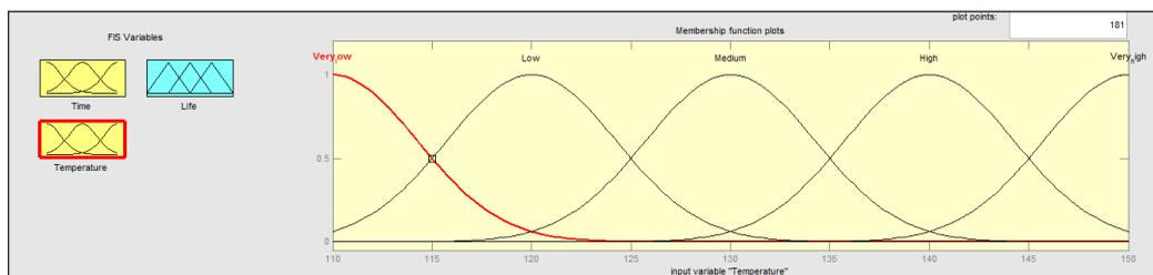
Figure 9. Gaussian membership functions for temperature
