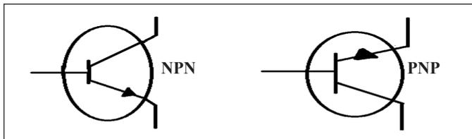
Figure 1. Symbol of bipolar junction transistor
