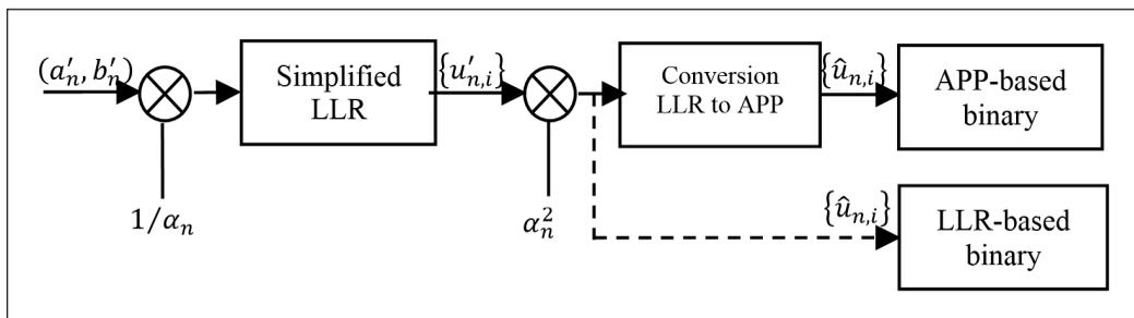
Figure 2. Principle of simplified APP calculation
