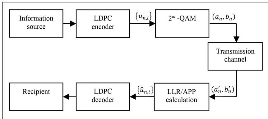
Figure 1. Diagram of a digital transmission system
