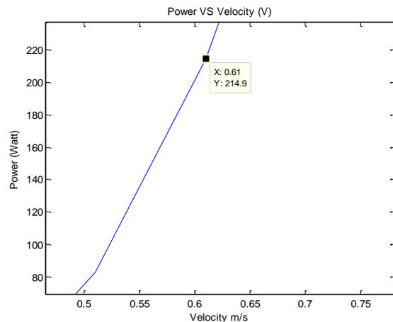
Figure 12: Power vs. Water Velocity
