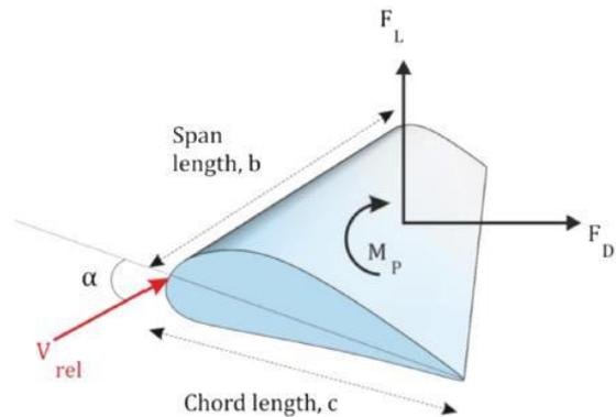
Figure 2: The resultant load on typical blade section [1].
