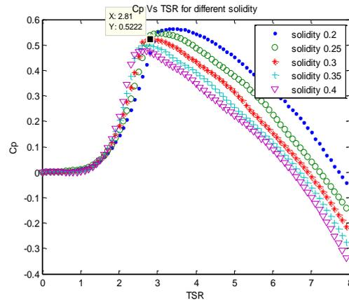
Figure 7: Power Coefficient at different solidity
