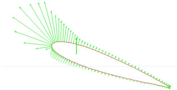
Figure 8: NACA0015 XFOIL analysis
