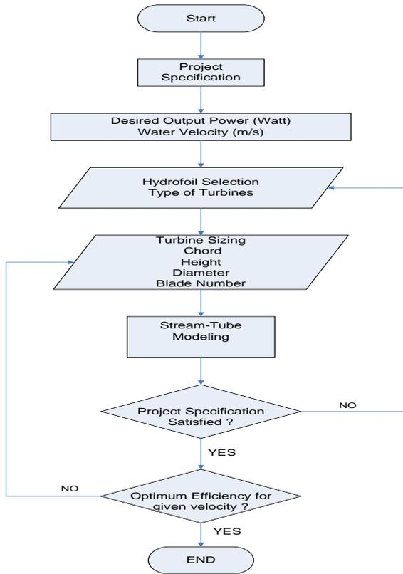
Figure 5: Design turbine flowchart
