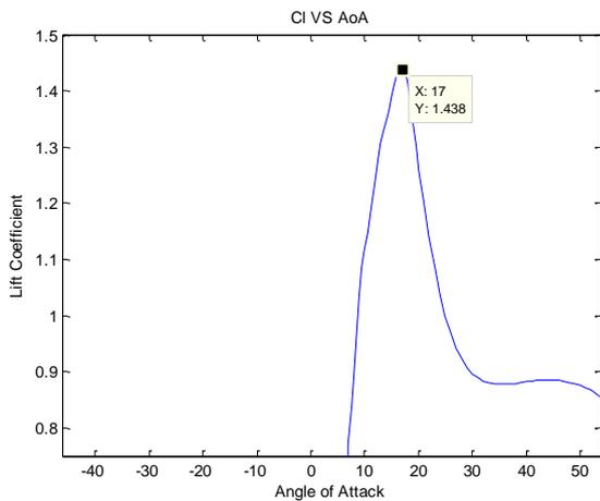
Figure 9: Lift Coefficient of NACA 0015
