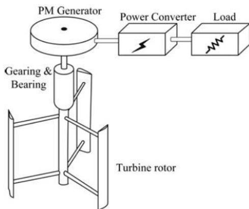
Figure 1: Vertical Axis Hydrokinetic System [11]
