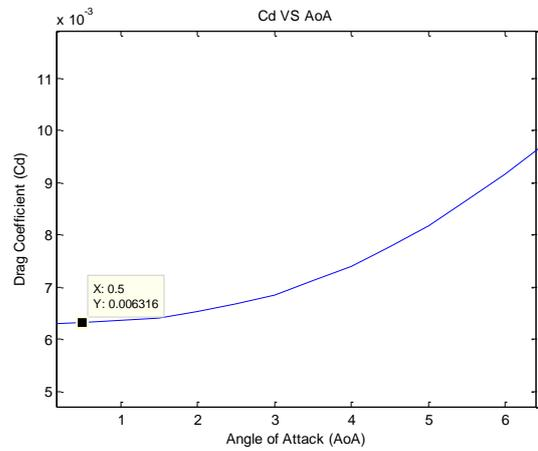
Figure 10: Drag coefficient of NACA 0015
