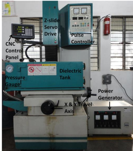
Fig. 2. Die sink EDM set-up.
