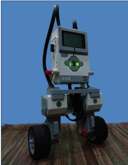
Figure 1: Two-wheeled balancing EV3 LEGO robot.
