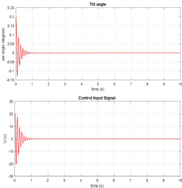
Figure 5: The tilt angle and control input signal (U) of the system using heuristic tuning method
