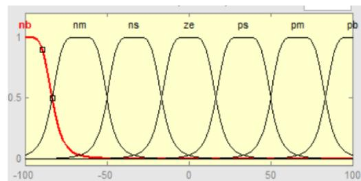
Figure 9: Input variable 'de/dt' for shape gbellmf 7 membership function
