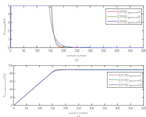
Figure 13: Step response of STFPID type Gaussian mf
