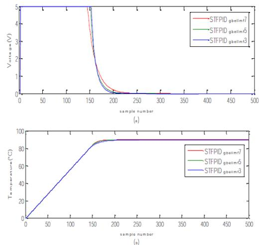
Figure 12: Step response of STFPID type Generalized bell mf
