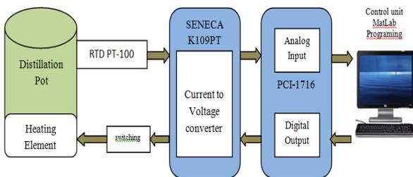
Figure 2: Block diagram of the induction-based steam distillation system
