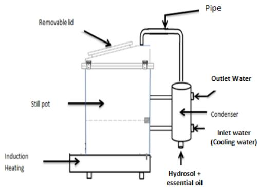
Figure 1: Sketch of steam distillation process for essential oil extraction
