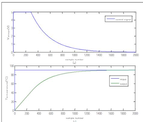
Figure 11: Step response for PID controller
