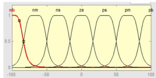
Figure 8: Input variable 'e' for shape gbellmf 7 membership function
