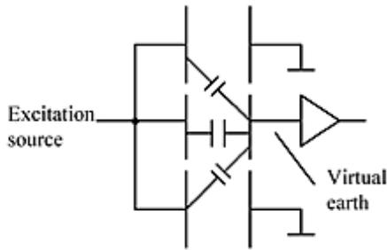
Figure 2: Connection of driven guard electrode.
