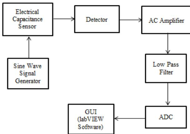
Figure 3: Block diagram of the complete system.
