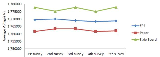
Figure 7: Average output voltage of FR4, Paper and Plastic.
