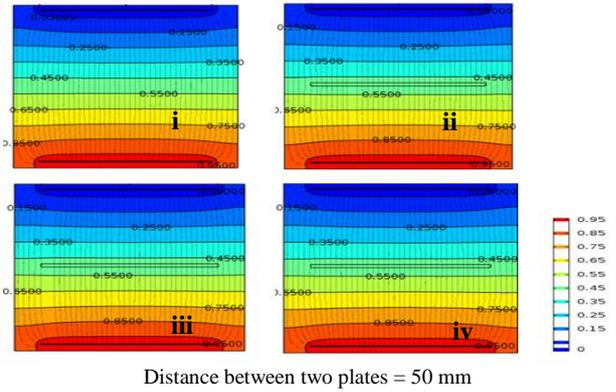
Figure 6: Contours of electrical potential and electric field lines when electrode 1 is excited on (i) air (ii) FR4 (iii) Paper (iv) Plastic
