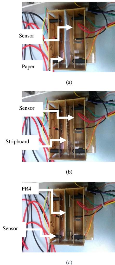
Figure 12: Material under test by Electrical Capacitance Sensor (ECS)
