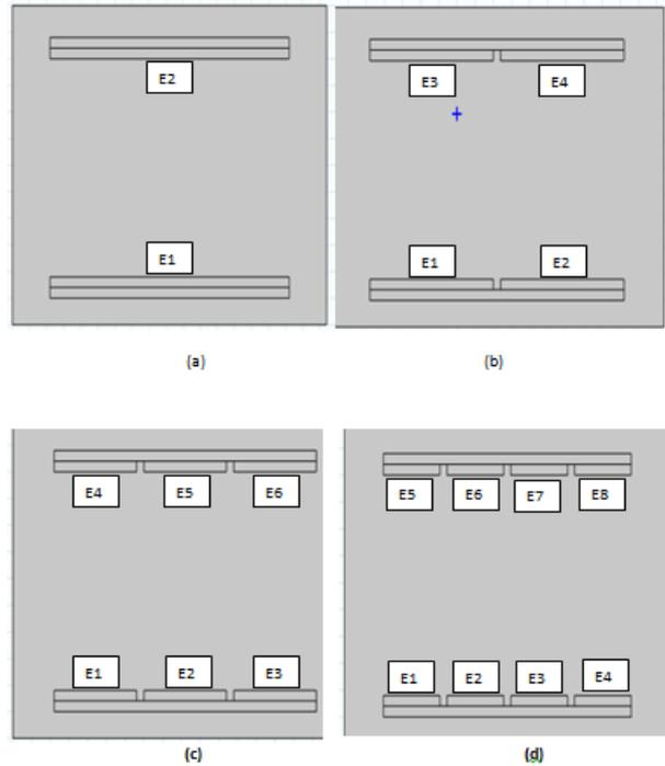
Figure 4: 2D models for parallel two plates ECS sensors. (a) Sensor with 1 electrodes (b) Sensor with 2 electrodes (c) Sensor with 3 electrodes (d) Sensor with 4 electrodes.
