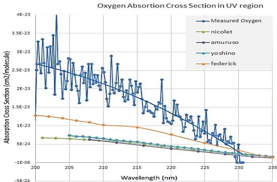
Figure 3: Oxygen absorption cross section spectrum between 200 nm and 230 nm.
