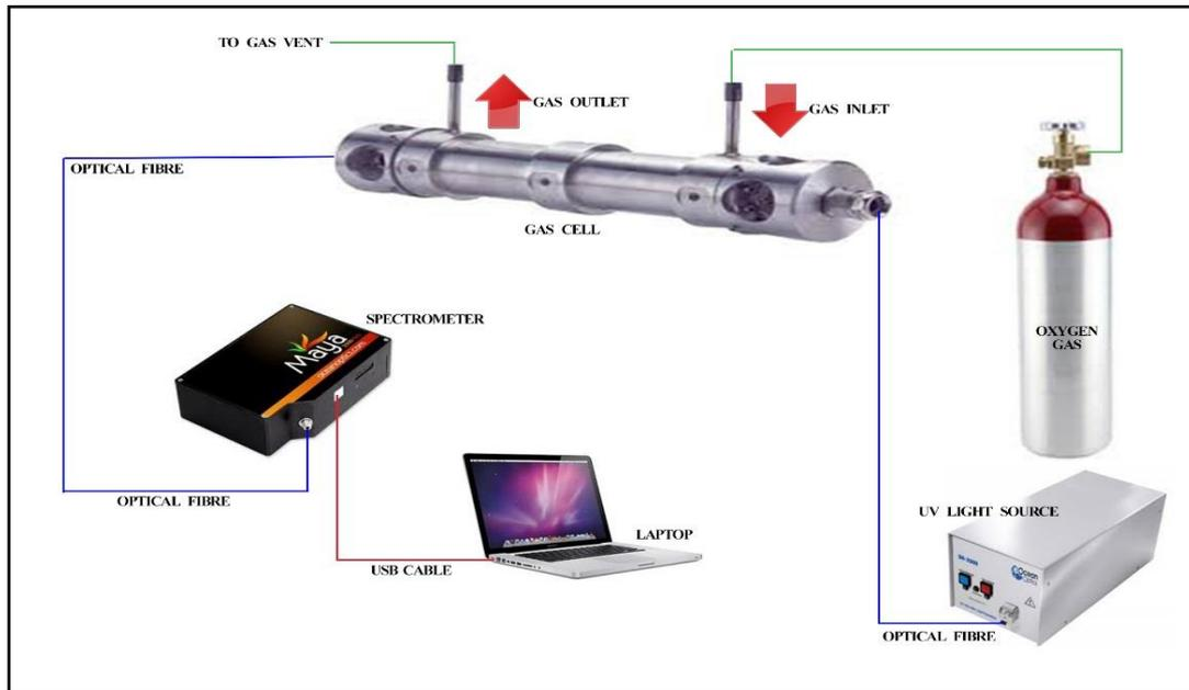
Figure 2: Generic design of Oxygen Detection System
