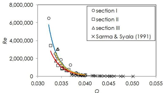
**Figure 7** Relationship between Reynold number and channel resistance at the outer bank comparing to the experimental result
