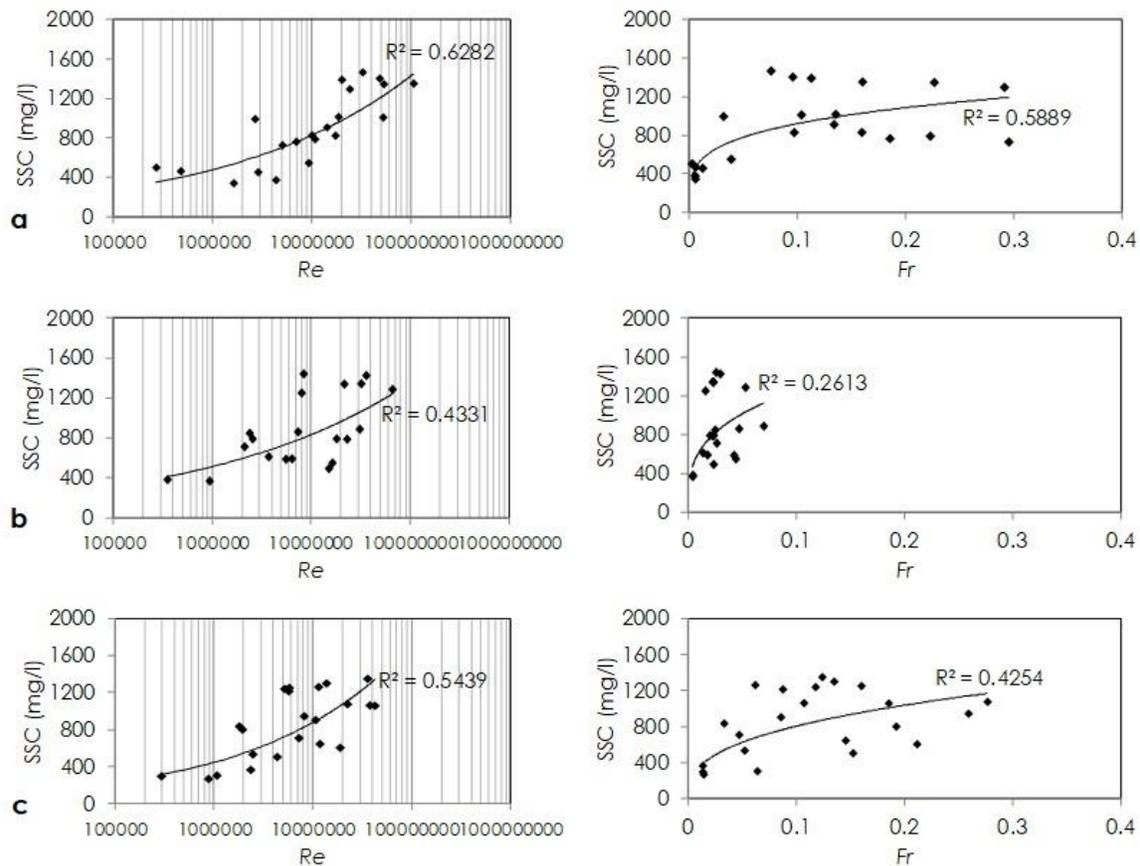
**Figure 6** SSC and flow parameter correlation at the outer banks of Cross section I (a), Cross section II (b) and Cross section III (c)
