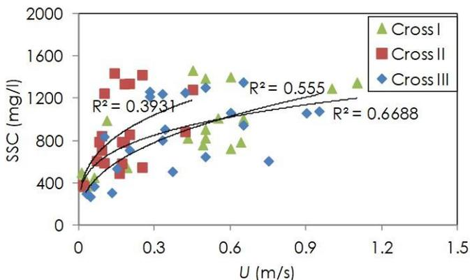
**Figure 5** SSC and flow velocity behavior at the outer bank of cross section I, II and III
