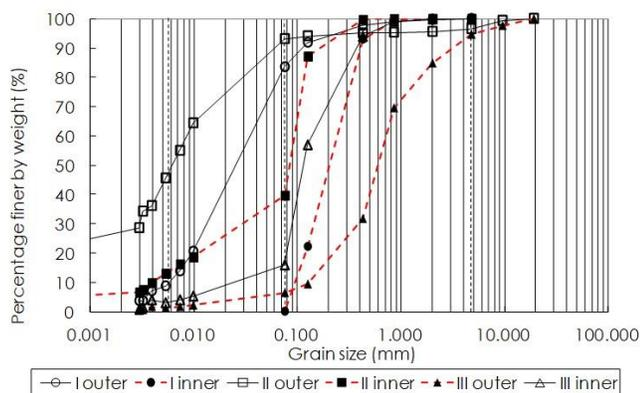
**Figure 3** Grain size distribution of bed material at inner and outer sections of study area
