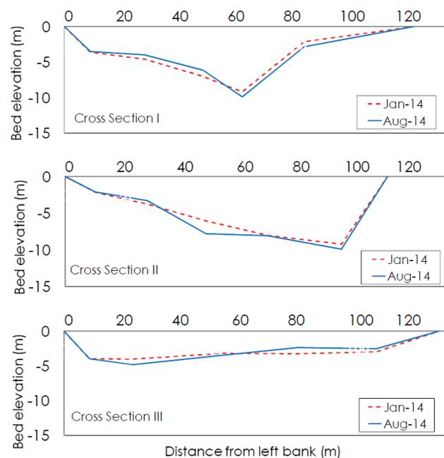
**Figure 4** Channel geometry changing at three cross sections between January and August 2014
