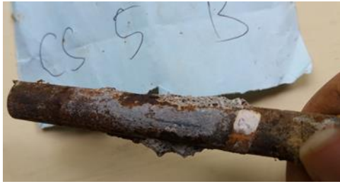
Fig. 5. Corrosion product on steel bar.
