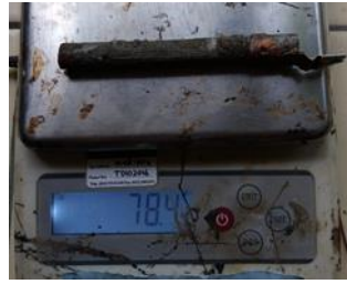
Fig. 6. Corrosion-free steel bar.
