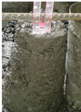
Fig. 7. Slump of conventional concrete.
