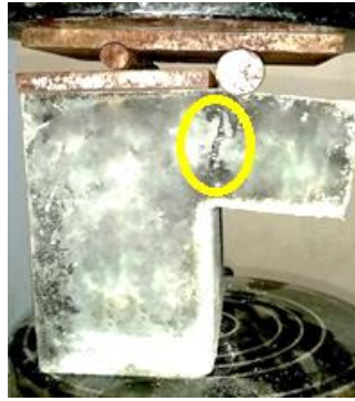
Fig. 5. Shear strength test specimen after failure with crack in the shear plane.
