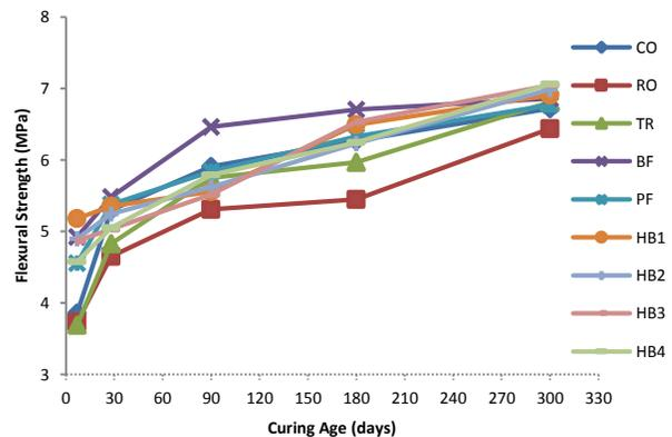
Figure 5 Flexural strength of tested specimens at various curing ages
