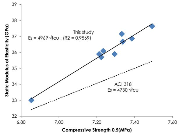
Figure 7 Relationship between  $E_s$  and square root of the compressive strength of concrete
