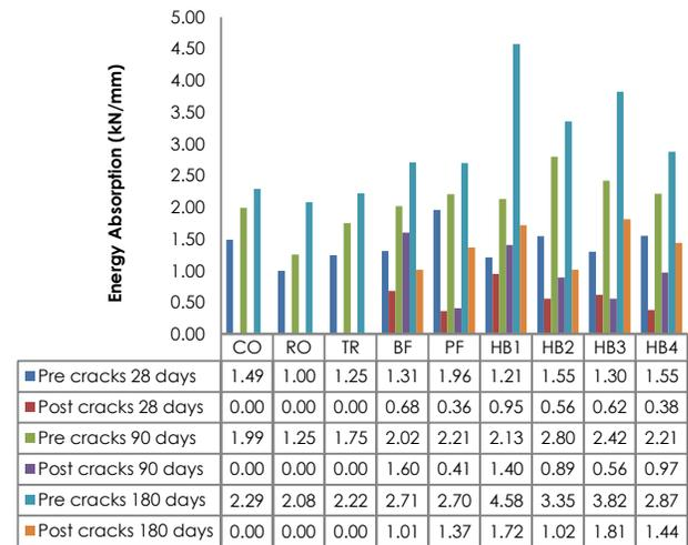
Figure 12 Pre-crack and post-crack energy absorption of all specimens exposed at various testing ages
