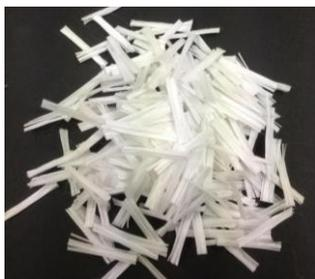
Figure 2 Fibrillated polypropylene fiber
