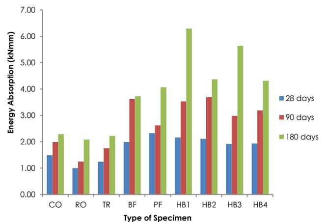
Figure 13 Total energy absorption of all specimens at various ages
