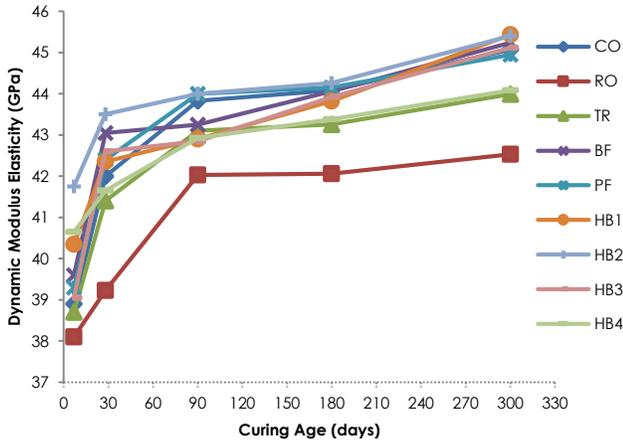
Figure 8  $E_d$  of tested specimens at various curing ages
