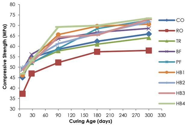
Figure 4 Compressive strength of tested specimens at various curing ages
