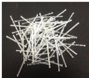
Figure 1 Polyolefin fiber
