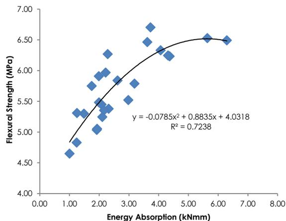
**Figure 14** Relationship between static flexural strength and impact energy of specimens
