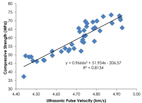
Figure 11 Relationship between UPV and compressive strength of specimens
