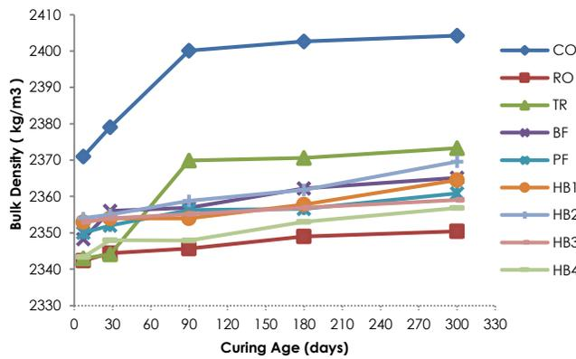
**Figure 3** Bulk densities of concrete specimens at various curing ages
