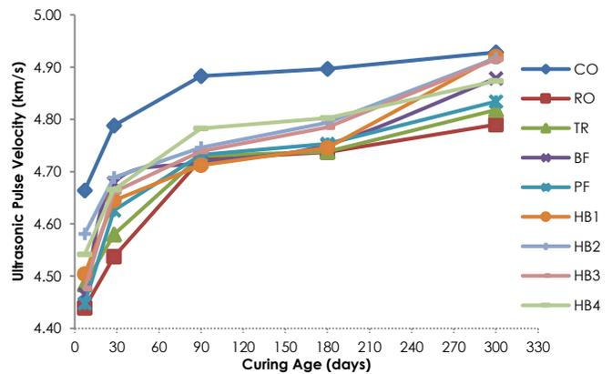
Figure 10 UPV of tested specimens at various curing ages
