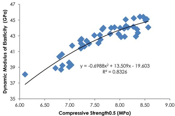
Figure 9 Relationship between  $E_d$  and compressive strength of specimens
